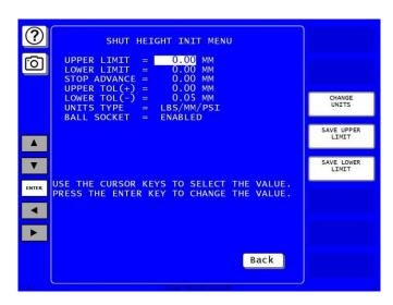
Figure 3-6. Shut Height Initialization Menu
