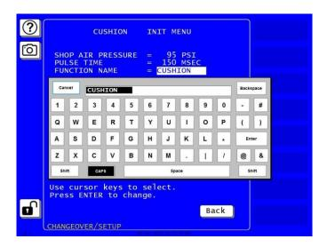
Figure 3-13. Cushion Control Initialization Menu with Entry Window Displayed
