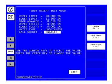
Figure 3-9. Shut Height Initialization Menu Completed
