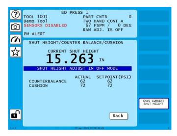
Figure 3-20. Shut Height/Counterbalance/Cushion Run Screen
