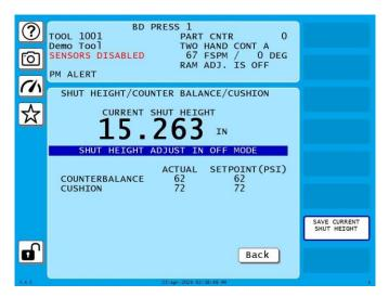
Figure 4-5. Shut Height/Counterbalance/Cushion Run Screen
