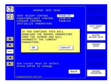
Figure 2-23. RamPAC Initialization Menu with Restore Parameters Warning Message
