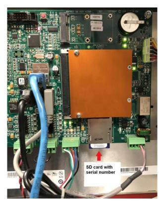
Figure 2-21. SmartPAC PRO SD Card with Serial Number on HMI Board
