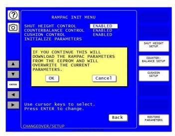
Figure 3-5. RamPAC Initialization Menu with Initialize Parameters Warning Displayed
