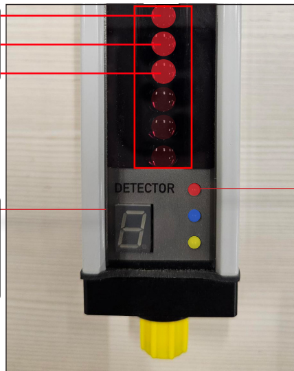
Shadow®10 LED Indicators and 7 Segment Display
