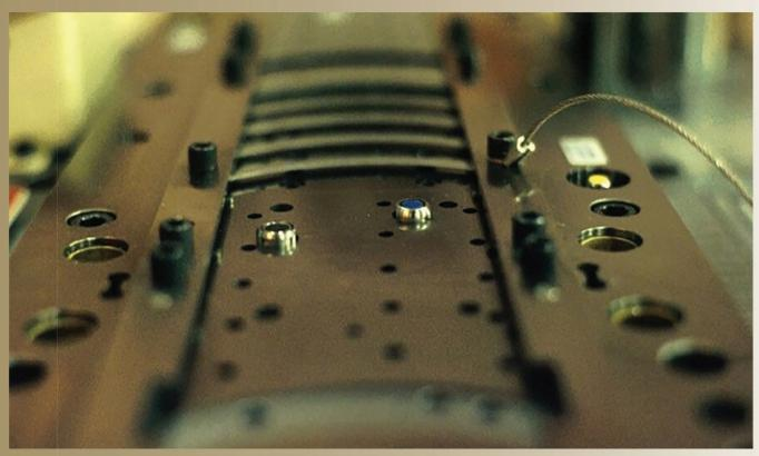
The best way to ensure that a sensor will work in the die is to try it out on the bench first.
