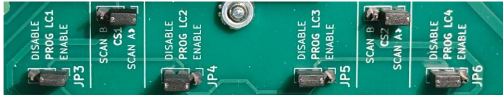
Figure 5-2. Jumpers JP3 – JP6, showing JP3 in the Enable Position
